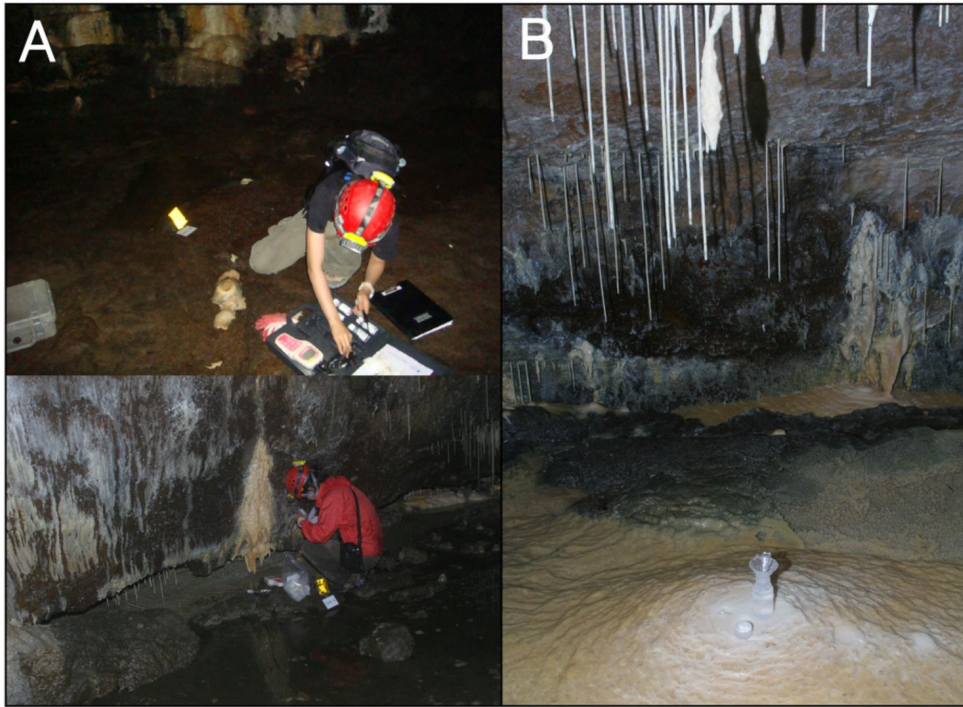
Figure 6. A) Monitoring sites for cave water conditions. B) Water sampling from dripping water.
